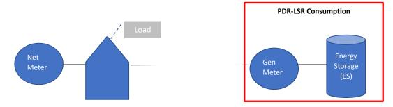
2. The PDR-LSR with Baseline is used when the facility load is offering load curtailment, and the behind-the-meter storage provides both load curtailment and load consumption. The facility load nets out the energy storage device and utilizes the customer load baseline to calculate load curtailment. The behind-the-meter storage will utilize the PDR-LSR curtailment calculation to combine the facility load CLB derived value. The PDR-LSR consumption will only apply to the behind-the-meter storage.
